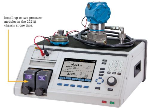
Use the 2271A to perform closed loop, fully automated calibration on 4--20~mA devices like this transmitter.
