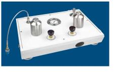
separation. Driven by a pneumatic pressure source (nitrogen bottle) and controlled by needle valves, high pressure gas is balanced against the liquid in a hydraulic deadweight tester through a series of fluid traps.
