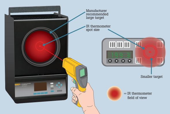
Infrared thermometers have peripheral vision.
