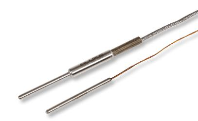
The 5606 and 5607 Full Immersion PRTs are designed to perform in extreme environments where both the transition minimum immersion depthjunction and the lead wires are required to withstand temperatures covering the entire operating range of the probe. ("Immersion" in this case simply means exposure to temperatures other than ambient and does not necessarily refer to the medium to which the PRT and its components are subjected.)
